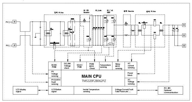
Sections marked with broken line indicate the inner aspect of the inverter.
